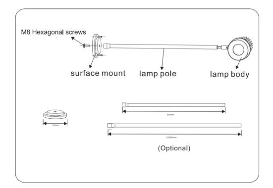
Step3: Merge the lamp part and the surface mout and using M8 Hexagonal screws to fix the surface mount..
